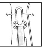
Squeeze the buttons (A) on the sides of the height adjuster and move the height adjuster to the desired position.
